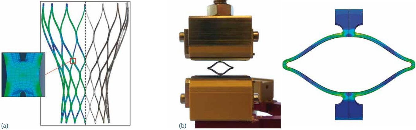
(a) Finite element analysis of a heart valve frame with a close-up view of a strut intersection. (b) Mechanical fatigue testing (left) helps correlate the results of FEA strain sampling (right).
